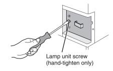
**NOTE:** Make sure the lamp unit and screw are installed securely; otherwise, the TV may not turn on and the lamp life may be shortened.
